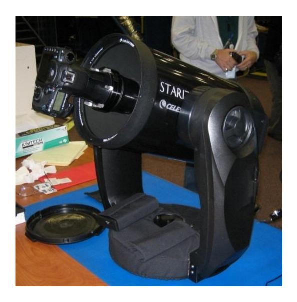
The ISERV camera, once on the space station, will be positioned to look through Destiny's Earth-facing window. ISERV will receive commands from Earth and acquire image data of specific areas on the Earth the next time the station passes over the region
