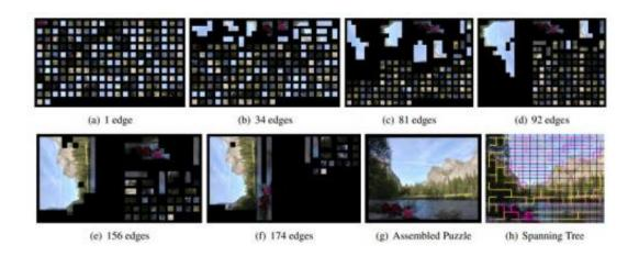
Puzzle assembly begins with each jigsaw piece as its own forest. Forests are merged (by combining and rotating, if necessary) to create assembled subclusters according to the compatibility score that we introduce (MGC), until the puzzle is assembled (a)-(g). The spanning tree in (h) shows the final representation of the solution as well as the order in which edges were added, from early (magenta) to later (yellow). This example has 192 jigsaw pieces. Image: Andrew C. Gallagher
