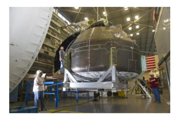
Fabricated at Alliant Techsystems in Iuka, Miss., the CCM was constructed in two parts using a hand layup technique, which combines carbon fiber epoxy and an aluminum honeycomb core. The two parts were joined together and then bonded in a unique process developed at
