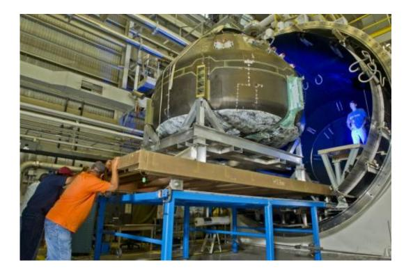
The Composite Crew Module being rolled into the vacuum chamber at Marshall's Environmental Test Facility. The test will continue through the end of the summer. Credit: NASA/MSFC/Emmett Given
