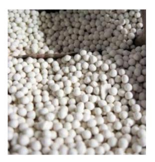
These zeolite pellets can bind steam within their pores, generating heat. Credit: Fraunhofer IGB
