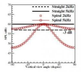
Simulated beam patterns of straight and spiral cochleas: While the straight cochlea generates beam patterns without any vertical variation, the spiral cochlea generates beam patterns that vertically localize the sound source. Image credit: Xun Huang, et al. ©2012 EPLA
