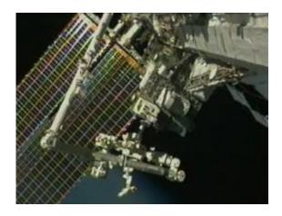
RRM (center, on platform) uses Canadarm2 and the Canadian Dextre robot (left and bottom, foreground) to demonstrate satellite-servicing tasks. Credit: NASA/CSA
