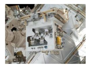
The Robotic Refueling Mission (RRM) module on the International Space Station before it was installed on its permanent platform. Credit: NASA
