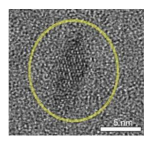
This image from an electron microscope shows a coated titanium dioxide nanocrystal. Credit: Joel Schrauben/James Mayer/UW
