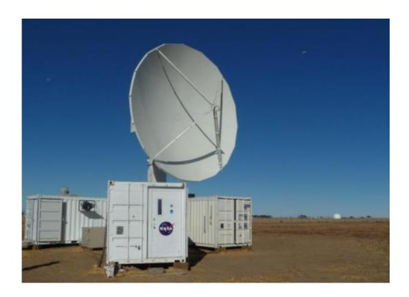
The NASA NPOL radar is a research grade S-band, scanning dual-polarimetric radar. It underwent a complete antenna system upgrade in 2010 and is one of two fully transportable research-grade S-band systems in the world. It is used to make accurate volumetric measurements of precipitation including rainfall rate, particle size distributions, water contents and precipitation type. Credit: NASA
