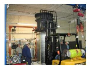
Researchers and staff at UT's Magnet Development Laboratory prepare the central solenoid mockup for the vacuum pressure impregnation process. Credit: University of Tennessee, Knoxville
