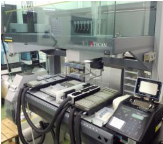
Figure 1: The automated CAGE cDNA preparation system for rapid genome-wide gene expression analysis. © 2012 Masayoshi Itoh, RIKEN Omics Science Center
