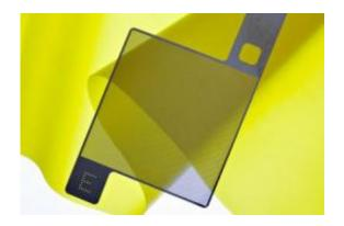
This image shows the lattice-shaped electrode in the foreground, and the elastomer in the background. Credit: This image shows the lattice-shaped electrode in the foreground, and the elastomer in the background.
