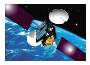
Artemis, an artist's impression. Carrying three payloads plus a number of experiments, ARTEMIS (Advanced Relay and Technology Mission Satellite) is being developed for testing and operating new telecommunications techniques. Credits: ESA - J. Huart
