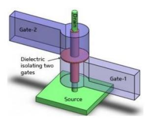
The nanowire transistor uses two wrap-around metal gates to define two distinct transistors on a single nanowire (vertical rod). Credit: 2011 IEEE
