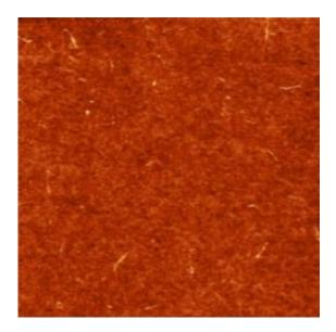
An atomic-force microscope image of a layer of single-walled carbon nanotubes deposited on a silicon surface, as the first step in manufacturing the new type of solar cell developed by an MIT team. Individual nanotubes can be seen in the image. Photo: Rishabh Jain et al
