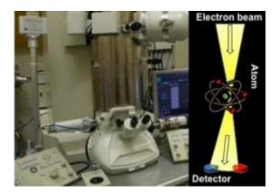
The scanning transmission electron microscope used in the experiment and a conceptual depiction of the new technique.
