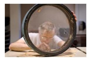
Augustine spent several days disassembling and cleaning the achromatic doublet lens, an assembly that weighs an estimated 50 pounds, using a series of distilled water baths and small brushes to free the elements of accumulated dust, debris and the occasional mud wasps' nest. Credit: Jeff Miller
