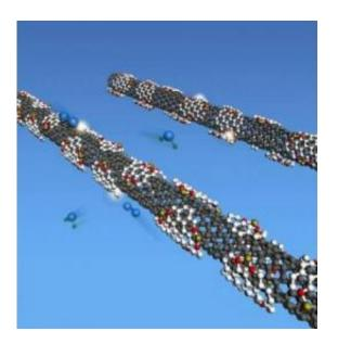
This drawing shows the damaged outer wall of a carbon nanotube with nanosized graphene pieces (white patches), which facilitate the formation of catalytic sites made of iron (yellow) and nitrogen (red) atoms. The catalyst reduces oxygen to water. Credit: Guosong Hong
