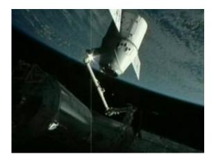
In this frame grab from a NASA video, the robotic arm of the International Space Station holds the SpaceX Dragon capsule on May 25 as astronauts prepare to dock the capsule with the station. The capsule is preparing to make its return journey to Earth.
