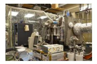
A SURF beam line (foil-wrapped cylinder at right) ends at a vacuum chamber in which the MAVEN EUV filter radiometer was tested. At left, plastic drapes form a clean room in which the instrument can be extracted from the chamber and from its mounting hardware.
