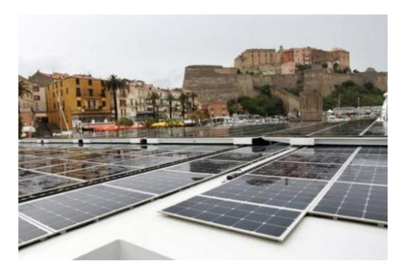
The are 537 square metres of black solar panels mounted around a raised cockpit aboard PlanetSolar. Planetsolar can produce up to 500 or 600 kiloWatts per hour in good weather -- enough to travel 300 km when the battery is fully charged using engines no more powerful than those on a scooter.
