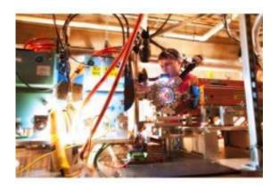
SLAC graduate student Spencer Gessner aligns a mirror for FACET's X-ray spectrometer. The instrument was just one of the many new instruments and pieces of equipment installed in the beam tunnel to turn part of a 50-year-old linear accelerator into a new user facility. Credit: Brad Plummer
