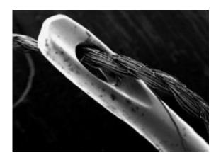
Scanning Electron Micrograph (SEM) of needle and thread. Credit: Public Domain Image
