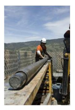
Ryan O'Grady of LacCore examines a 3-meter coring tool after it's brought up from 137 meters below the bottom of Clear Lake. The tool contains a plastic pipe that encases the lake sediments. Credit: Robert Sanders, UC Berkeley media relations
