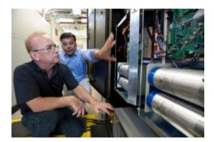
NREL engineers Sudipta Chakraborty and Bill Kramer examine the design of the power block at an NREL lab. Along with an industrial partner, NREL engineers have developed the power block for renewable and distributed energy applications. Credit: Dennis Schroeder
