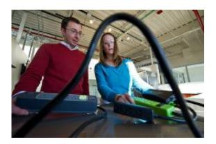
NREL engineers Dane Christensen and Bethany Sparn test advanced power strips at NREL's Automated Home Energy Management Laboratory. The lab enables researchers to study the complex interactions of appliances and other devices in connection to the energy grid. Credit: Dennis Schroeder
