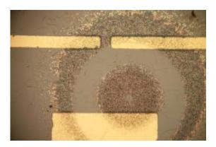
Gold electrodes rest on clumps of vanadium oxide (VO2) wires that are each about 1,000 times smaller than a human hair. When baked in the presence of hydrogen gas, the wires next to the electrodes (dark region) absorb hydrogen and exhibit altered electronic behavior. CREDIT: Jiang Wei/Rice University
