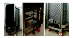
This shows a rack unit. (Left) The front view of the rack structure is fully stacked with trays in tilted position. (Center) This shows the detail of the endless screw jack system and its hand wheel controller. (Right) The back view shows the bottom frame of the rack with the plastic curtain, the metallic slide and the basket collector. Credit: © 2012 Entomological Society of America
