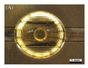
A drop of liquid sits on the textured silicon surface that has arced rungs to guide the drop, and a grid of pillars to keep the drop in the channel. Credit: Karl Bohringer, UW
