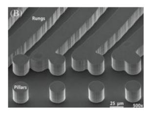
This is a close-up of the UW surface showing the arc edges and adjacent pillars. Credit: Karl Bohringer, UW
