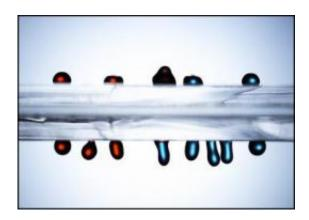
Drops of red and blue liquid move along the upper and lower surface of the vibrating UW platform at speeds up to 1 inch per second. This combined image shows drops as they move toward the center and merge. Credit: Karl Bohringer, UW
