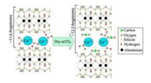
Like a confused dieter, the common clay montmorillonite would plump up, but nobody knew why. Scientists at Pacific Northwest National Laboratory showed that the clay grows because carbon dioxide molecules from the supercritical CO2 work their way into the mineral, making it expand.
