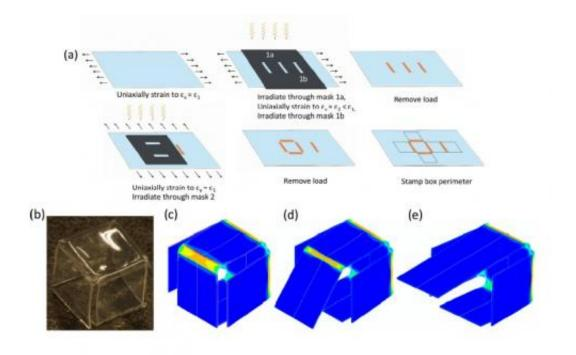
A six-sided box fabricated by photo-origami is constructed by straining and irradiation to form hinges. (a) The photo-origami protocol; (b) a fabricated closed box; and (c), (d), and (e) a simulated box with closed, partially open, and open tops. Image caption: Ryu, et al. © 2012 American Institute of Physics
