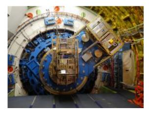
The GREAT far-infrared spectrometer is mounted to the telescope flange, inside the pressurized cabin. During observations GREAT rotates  $\pm 20$  degrees from the vertical. R. Güsten
