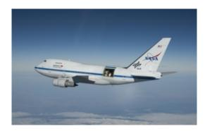
SOFIA, the "Stratospheric Observatory for Infrared Astronomy" cruises above Southern California with its large cavity door wide open; the 2.7-meter Germanbuilt telescope is visible. At altitudes of up to 45000 ft the observatory operates above 99.8% of the atmospheric water vapor. Credit: NASA
