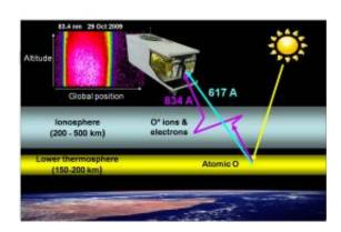
This image shows a schematic representation of the dayside ionosphere remote sensing concept, using measurement of the scattered 83.4 nm emission to infer ionospheric densities. Measuring the 61.7 nm emission provides direct information on the intensity of the source region in the lower thermosphere that is currently only modeled for operational algorithms. Credit: U.S. Naval Research Laboratory
