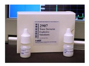
The new NIST reference material for explosive traces contains meticulously measured concentrations of the explosives TATP and PETN. The material can be used to test and validate the ability of machines and methods to detect the explosives' presence. Credit: Talbott/NIST
