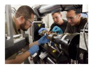
NASA scientists Santo Padula (left) and Othmane Benafan (right) and Central Florida University student Doug Nicholson are using the VULCAN instrument at SNS to study the atomic-level structure and behavior of shape-memory alloys such as nickel titanium. Their aim is to create more robust SMAs that can be commercialized for aerospace and other uses.
