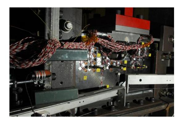
Load-withstanding capabilities of the Orion service module's conical adapter joint are tested at Marshall's Material Environment Test Complex facility. The test was successfully completed in March. Credit: NASA/MSFC
