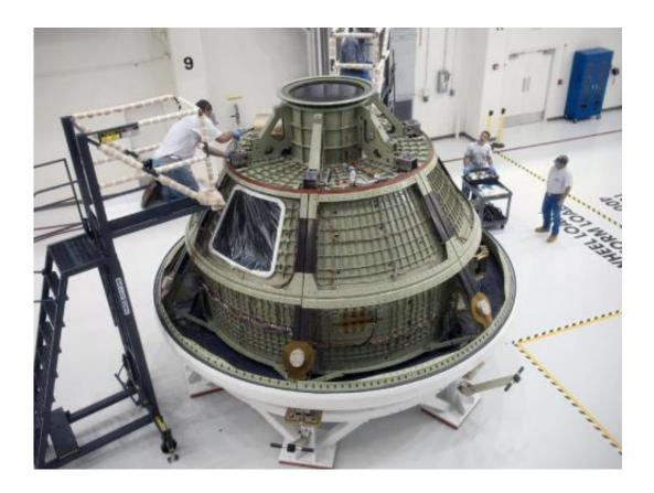
The Orion Ground Test Vehicle shows the Orion "skeleton" used for pathfinding operations in preparation for the Orion spaceflight test vehicle slated for NASA's Exploration Flight Test, or EFT-1, in 2014. Credit: NASA
