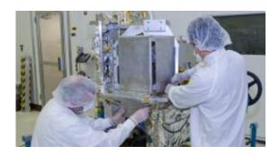
Technicians prep the OCO-2 instrument for shipping at JPL. The instrument consists of three parallel, high-resolution spectrometers, integrated into a common structure and fed by a common telescope. Image credit: NASA/JPL-Caltech
