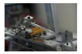
The mechanical IV DRIP invented by students at Rice University takes cues from mousetraps for its ability to halt the flow of fluid through an intravenous line without electricity. (Credit: Jeff Fitlow/Rice University)
