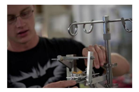
Thor Walker attaches a line to the IV DRIP device created by a team of freshman engineering students at Rice University. A counterweight lowers as the IV bag gets lighter and trips a shutoff mechanism at the right level. (Credit: Jeff Fitlow/Rice University)
