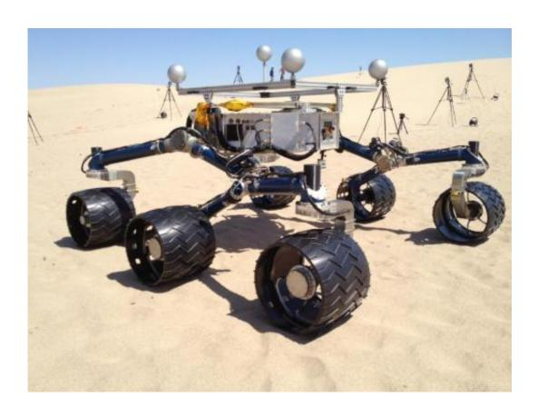
Mars Science Laboratory mission team members ran mobility tests on California sand dunes in early May 2012 in preparation for operating the Curiosity rover, currently en route to Mars, after its landing in Mars' Gale Crater. Credit: NASA/JPL-Caltech
