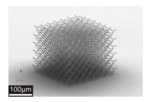
Pentamode metamaterials almost behave like fluids. Their manufacture opens new possibilities in transformation acoustics. Credit: Source: CFN, KIT
