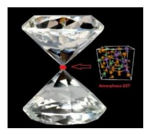
This illustration depicts the shape of diamond tips used to apply pressure that uncovered important new properties in the memory medium GST. The inset represents the atomic structure of amorphous GST. Credit: Ming Xu/JHU
