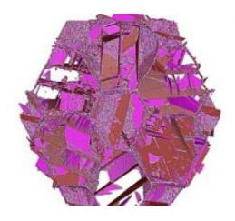
The image shows the simulation of a polycrystalline nanotwinned copper and its defects during tensile loading. Credit: 2011 Elsevier
