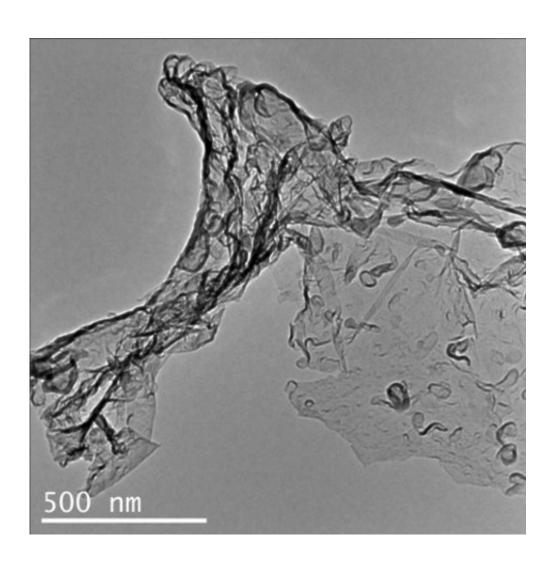
Transmission electron microscopy image of carbon nitride created by the reaction of carbon dioxide and Li3N.
