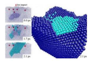
This shows a computer-model image of an island of metal atoms formed after bombardment by noble gas ions. Atoms disturbed by the bombardment cluster together under the surface and then glide back up in a matter of 2.1 trillionths of a second, or picoseconds. Credit: Kim Lab/Brown University
