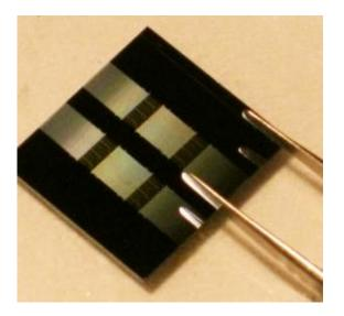
Researchers have now shown that quantum light sources can be fabricated using silicon, the most widely used material underpinning modern electronics. Shown here is a silicon photonic chip containing several dozen devices designed and fabricated by graduate students at the Electrical and Computer Engineering department at UC San Diego.
