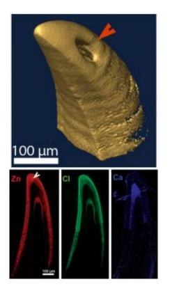
Above: A micro-computertomographic image of a fang tip. The orange arrow points to the opening of the venom canal. Below: The distributions of the metal ions zinc (red) and calcium (blue) and of chloride (green) are analysed using energy dispersive x-ray spectroscopy. Whereas the zinc and chloride are found in the outer layer of the fang, the calcium occurs in its interior. An increased concentration of zinc is also found in the centre of the fang tip. Credit: MPI of Colloids and Interfaces
