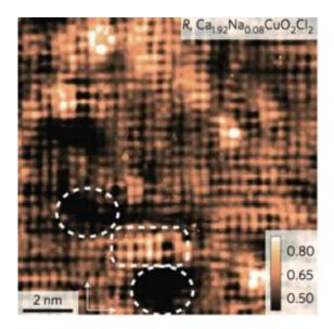
Scanning tunneling microscope image of a partially doped cuprate superconductor shows regions with an electronic "pseudogap" (rounded rectangle) others with no progress from the original insulator (dashed circles). As doping increases, pseudogap regions spread and connect, making the whole sample a superconductor.
