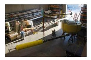
Mechanical technician John Ferreira prepares the power buoy for a deployment in MBARI's high bay. At this stage in the design process, the hydraulic piston was enclosed in a cylindrical housing of yellow foam (at lower left). Image: François Cazenave. Credit: 2011 MBARI
