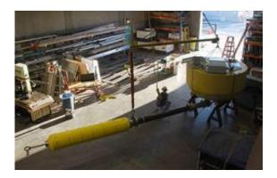
Mechanical technician John Ferreira prepares the power buoy for a deployment in MBARI's high bay. At this stage in the design process, the hydraulic piston was enclosed in a cylindrical housing of yellow foam (at lower left). Image: François Cazenave. Credit: 2011 MBARI
