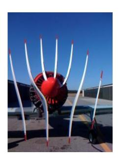
The rolling-shutter effect is a visual distortion and vertical shift of the centroid of a rotating propeller caused by the time delay from the horizontally-moving shutter of the camera.
