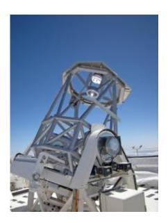
With a mirror diameter of 1.5 metres, an adaptive optics system and various instruments such as spectrographs and cameras, Gregor is one of the three most powerful instruments in the world for observing the sun. © Kiepenheuer Institute for Solar Physics
