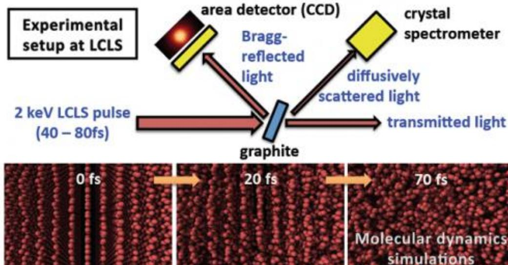
Demonstration of ultrafast disintegration of matter by 2 keV LCLS pulses: The team combined techniques commonly used in solid state physics (Bragg reflection) with techniques from plasma physics (spectroscopy of diffusely-scattered light) to characterize ultrafast heating in graphite.
