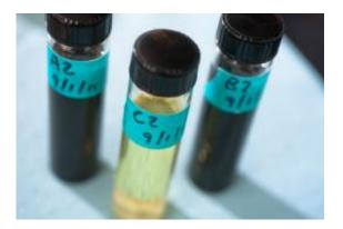
UB researchers are developing graphene-based anti-corrosion coatings. Here, three solutions for rust-proofing steel contain varying amounts of graphene.
