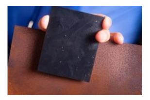
A graphene-based coating under development at UB keeps a piece of steel rustfree (foreground), in stark comparison with a rusted sheet of steel (background).
